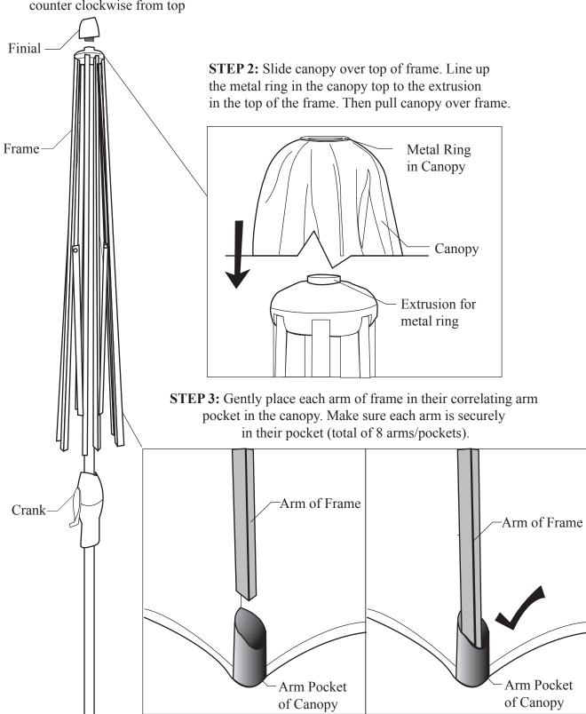
STEP 4: Reattach the finial by turning it clockwise into the frame extrusion.
