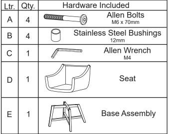
ASSEMBLY: Invert Seat (D) and align Base Assembly (E) over holes. Insert a bushing (B) followed by an Allen Bolt (A). Fully tighten using Allen Wrench (C). CAUTION: Hand tighten. No power tools.
