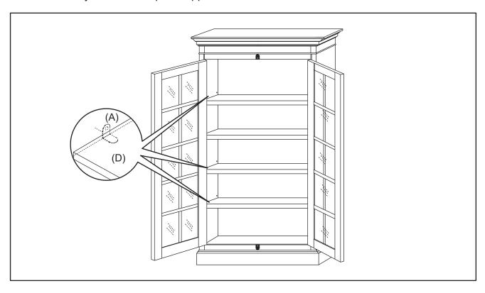
**LEVELERS**: Cabinet is equipped with Rotary Levelers under each corner, accessible from INSIDE Cabinet. Insert Flathead Screwdriver (not included) into opening and turn Leveler clockwise/counterclockwise to adjust. When complete, cover each opening with Wood Plug (B).
