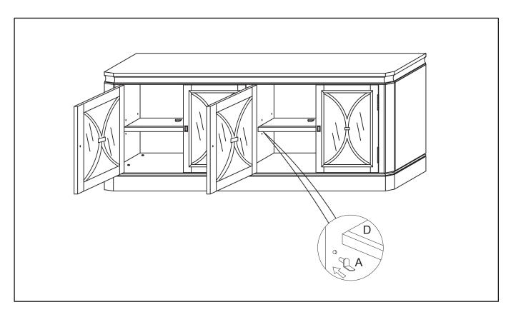
STEP 2: If the Console is uneven, adjust the levelers inside the bottom corners of the Console by using a flat head screwdriver. Turn clockwise or counterclockwise until the unit sits evenly. Cover the leveler holes the the wood plugs (C).
