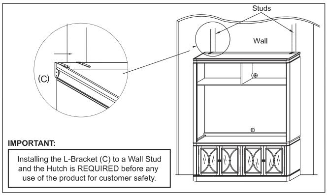
STEP 7: Pull the Hutch away from the Wall and attach the L-Brackets (C) to the Studs using the Long Screws (A).
