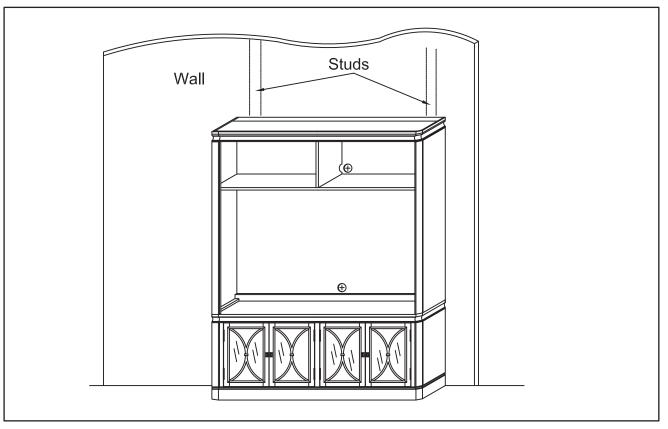
STEP 4: Slide the L-Bracket (C) over the top corner of the Hutch Top in front of the previously marked Stud and mark the Wall at the top of the L-Bracket.
