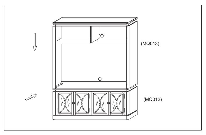
STEP 2: Align and set the Hutch (MQ013) on top of the Console (MQ012) . Attach the two Connector Plates (D) as shown using Connector Screws (E).
