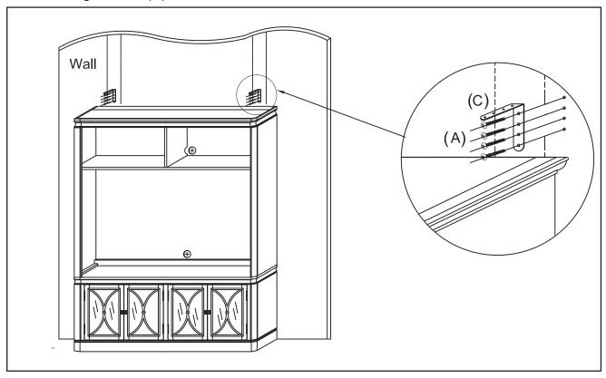
STEP 8: Slide the Hutch underneath the previously installed L-Brackets (C) and use 2 or more of the Small Screws (B) to attach the L-Brackets to the Hutch.
