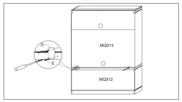
STEP 3: Center the Cabinet in front of two Studs and mark the Wall. Push the Cabinet against the Wall.
