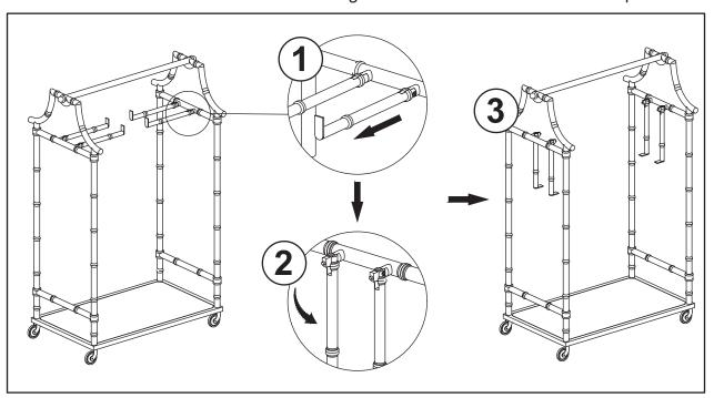
**ENGAGING HANGER RODS:** Pull up then pull out toward center, push back to lock in place.
