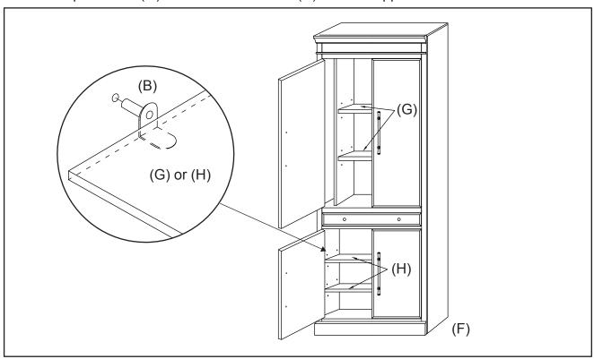
STEP 2: If the Cabinet Doors are uneven, adjust the levelers in the bottom corners inside the Cabinet (F) using a Flat head screwdriver. Turn clockwise or counterclockwise until the doors are even. Cover the leveler holes with the Wood Plugs (D). If the hinge screws are loose, use a Phillips head screwdriver to tighten them.
