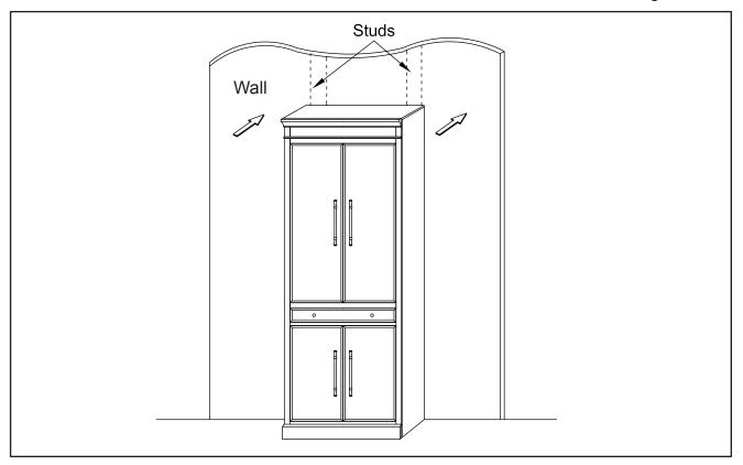
STEP 4: Slide the L-Bracket (E) over the top corner of the Cabinet (F) in front of the previously marked Studs and mark the Wall at the top of the L-Brackets.
