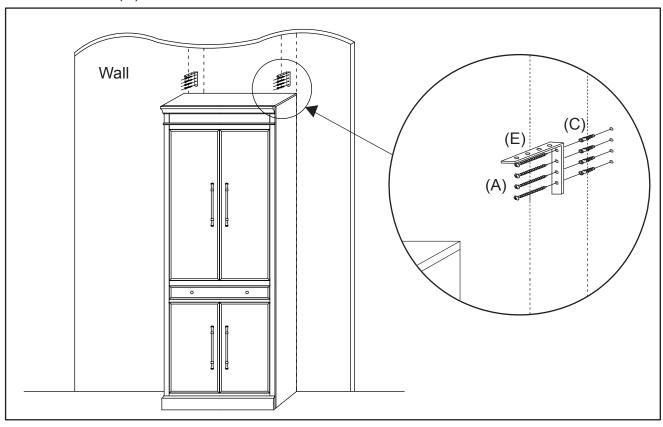
STEP 6: Slide the Cabinet underneath the previously installed L-Brackets (E) and use 2 or more of the Screws (A) to attach each L-Bracket to the Cabinet.
