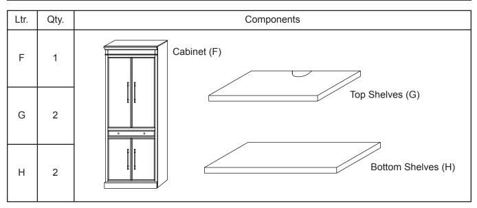
STEP 1: Place the Shelf Supports (B) at the desired Shelf heights in the Cabinet (F) and lay the Top Shelves (G) and Bottom Shelves (H) on the Supports.
