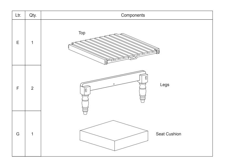
STEP 1: Attach the Legs (F) to the Top (E) using 4 90mm Allen Screws (A) and Allen Wrench (D). Then secure the Top (E) to the Legs (F) with 2 70mm Allen Screws (B) with the Allen Wrench (D).
