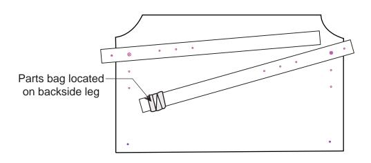
**STEP 1:** Place headboard face down on a clean surface. The 2nd screw has been installed at the factory. Straighten both legs so the predrilled holes line up with each other. The legs can be adjusted to 4 different heights to accommodate your mattress height. Feel for the holes (under the fabric) along the middle of the leg.Once you feel the holes and have figured out the height of your headboard, take a pair of scissors & cut a small hole over the necessary holes.
