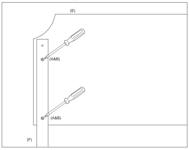
**STEP 3:** Attach the headboard to the bedframe. Place washer (D) on one of the screws (C) and insert it through the slots in your bedframe. Use the screwdriver to securely tighten the screw to the leg of the headboard. You will need to drill a pilot hole.
