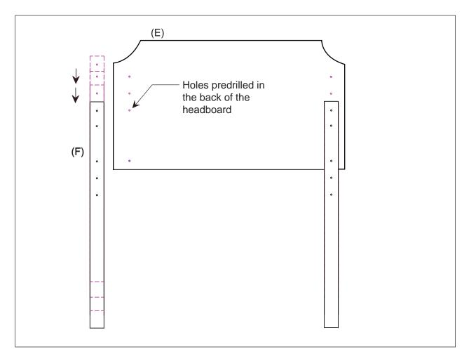
**STEP 2:** For each leg use one screw & washer in the top hole or 2nd hole, and the other screw and washer on the lower coordinating hole with a screwdriver.
