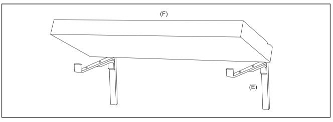
STEP 4: Center the Shelf on front of the Brackets (E). Attach the Shelf (F) and Bracket using the 3/4" Screw (D) in the Bracket front and the 1" Screw © at the back.
